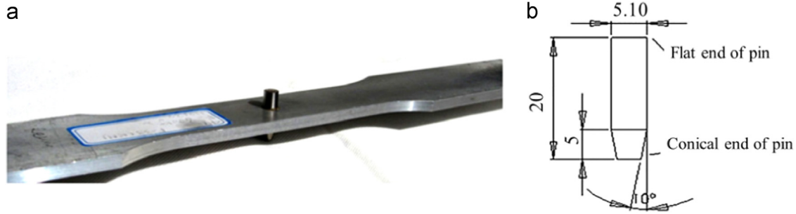
Fig. 3. The pin interference fitted specimens (a) and (b) the dimensions of pin for 2% interference fit [29].
